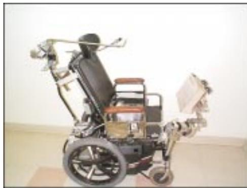
Figure 1: Deployed swing-away and communication board mounts.
