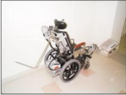
Figure 2: Stowed position of the swing-away and communication board mounting linkages.
