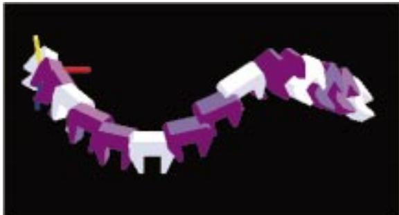
Figure 7: The end-effector trajectory is defined by interpolating key frames.
