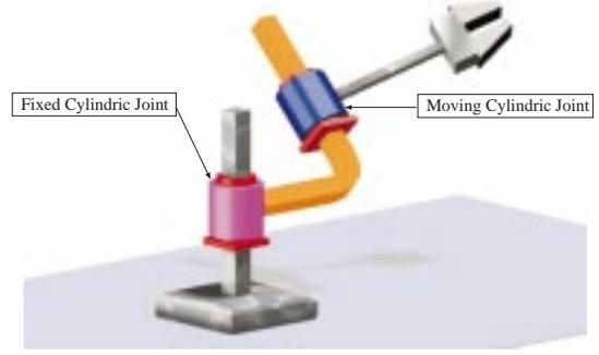
Figure 5: The CC open chain robot.
