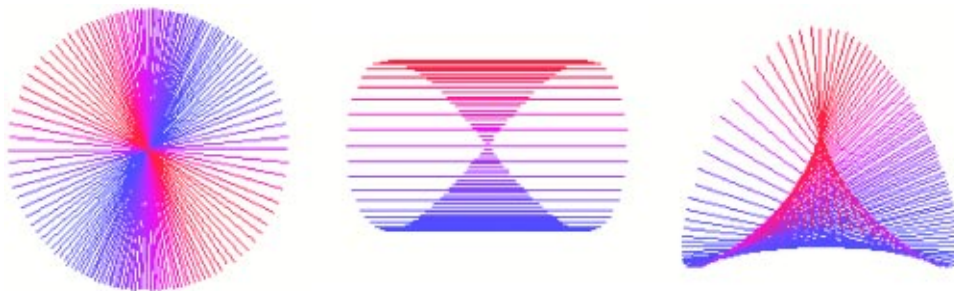
Fig. 3 The cylindroid as viewed first from the top along the central axis, then from the side and finally, from an angle
