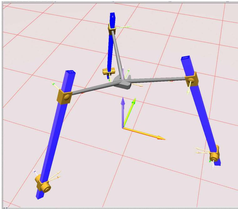
Figure 2: An RPS chain imposes one constraint, so a 3RPS spatial linkage has three degrees-of-freedom.
