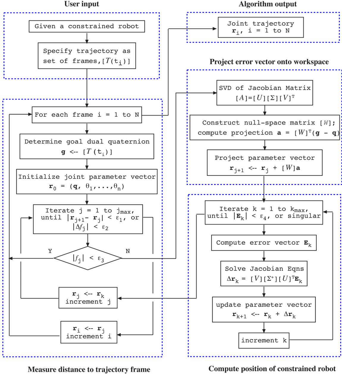
Figure 3: Flowchart of the trajectory generating algorithm.
