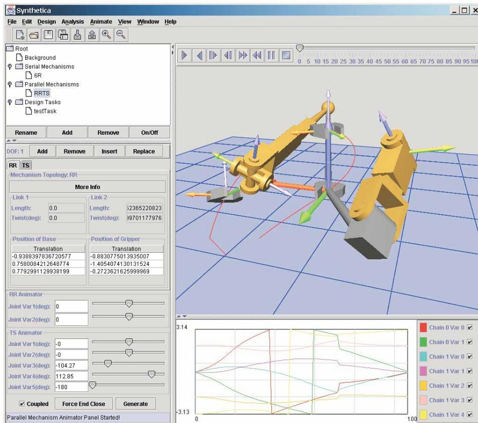
Figure 6: The user interface for the Synthetica software system.
