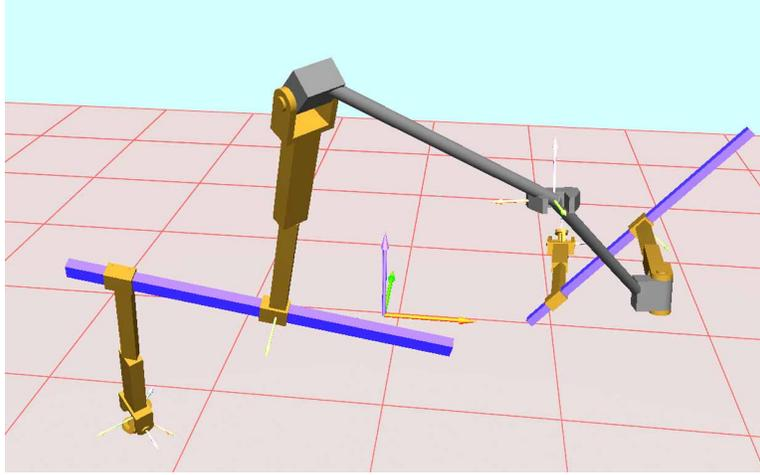
Figure 1: A TPR chain imposes two constraints, so a 2TPR spatial linkage has two degrees-of-freedom.
