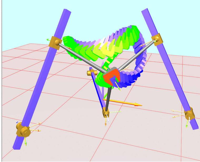
Figure 5: Example of the trajectory of a 3RPS linkage that approximates a specified movement.
