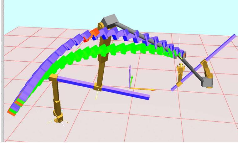
Figure 4: Example of the trajectory of a 2TPR linkage that approximates a specified movement.
