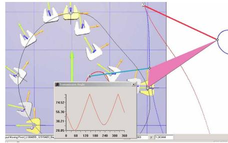
Figure 11: Alternative solution with better transmission angle
