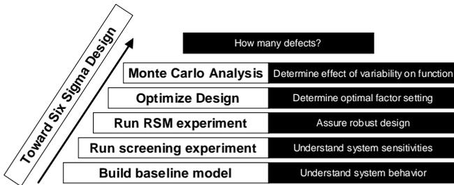
**Figure 1. Relationship between Six Sigma, Robust Design, and Design of Experiments**
