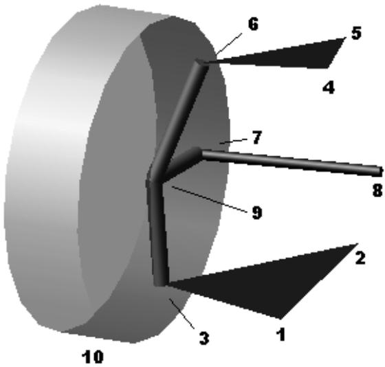
**Figure 1. ADAMS model of SLA suspension with numbered hardpoints corresponding to Table 1 (right side shown).**
