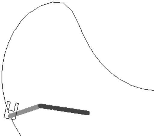
**Figure 3. ADAMS model of the ASME linkage challenge problem**
