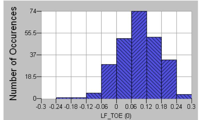
**Figure 5. Suspension toe angle histogram from Monte Carlo analysis**
