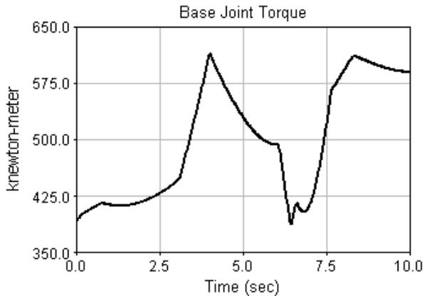
**Figure 4. Baseline torque magnitude on robot base joint.**
