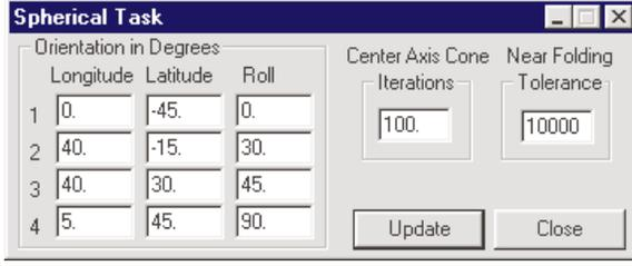
**Fig. 3.** The task of the linkage is defined by four orientations input through the Spherical Task dialog box.
