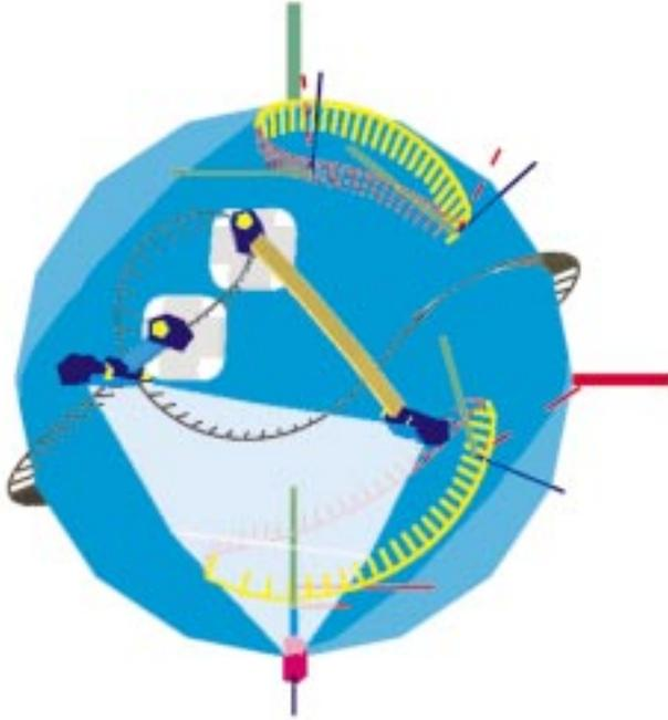
**Fig. 8.** The animation of a spherical linkage guiding its goal frame along a coupler curve is a useful evaluation tool.
